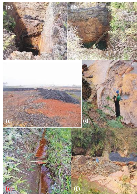
Fig 17 (a). Rat-hole mining- a crude mining technique (b) Mine shaft filled with rain water (c) Stockpiles of Coals (d) Corrosive layer seen on rocks at the river side (e) Drainage from stockpiles to nearby agricultural fields (f) Rat-hole mines at the river side
