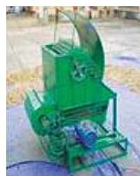
Fig 28. Modified power paddy thresher
